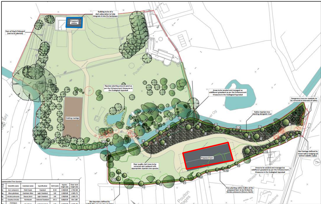
Figure 2: Site layout and proposed landscape enhancement. The proposed barn in red and stables in blue .
